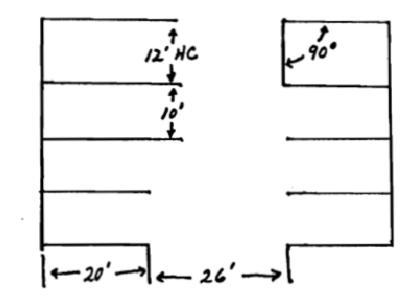
(2) Any off-street parking may be designed with access aisles with one way traffic. Access aisles with one way traffic may be reduced to sixteen (16) feet in width for 45 degree and 30 degree angle parking (See Figure 5).
