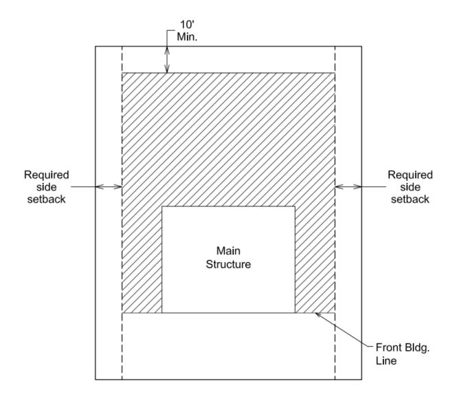
Figure 2. Allowable area for large accessory structures (> = 150 sf) on small (<1 acre) lots, and for all accessory structures on large (>= 1 acre) lots.
