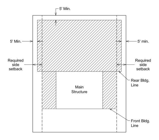
Figure 1. Allowable area for small accessory structures (<150 sf) on small (<1 acre) lots.
